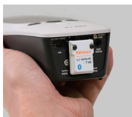
With Wireless Unit for Measuring Instrument U-WAVE-TIB installed
